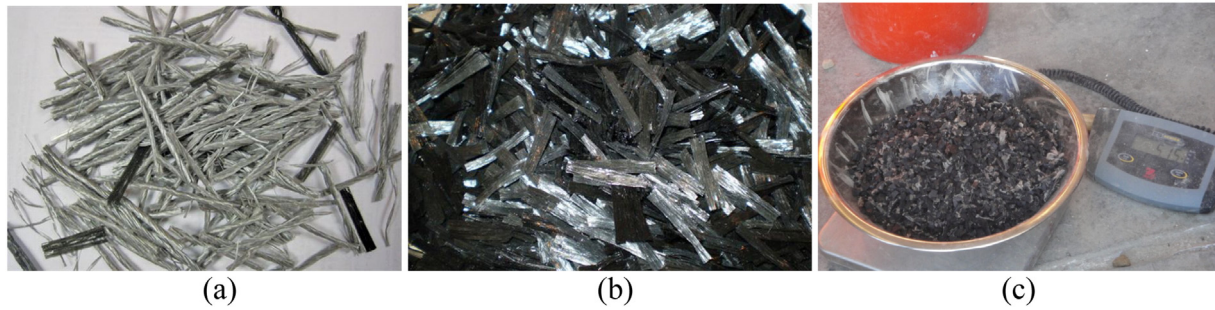
Fig. 1. Admixtures in permeable concrete: (a) Ferro-green fiber; (b) green-net fiber; (c) shredded tire chip.
